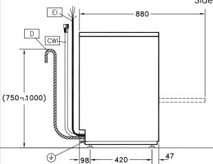
CWII Cold Water inlet 1 (cleaning) Drain ΕI Electrical inlet (power) EO **Electrical Outlet**
